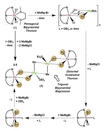
Scheme 1. Reaction of  ${\bf 1}$  with MeMgBr to form the fully brominated analogue of complex  ${\bf 3}$ .
