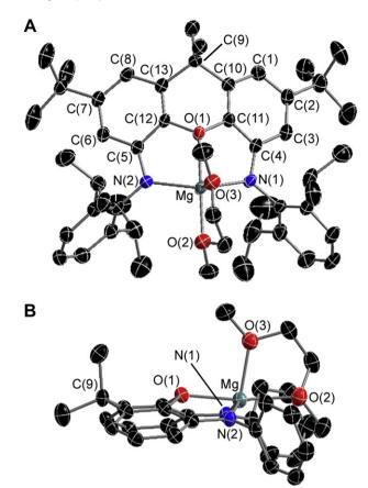
Fig. 3. The solid state structure of 6 hexane with thermal ellipsoids at 50% probability. Lattice solvent and hydrogen atoms are omitted for clarity. In view B, isopropyl and tert-butyl groups are also omitted for clarity. Selected bond lengths (Å) and angles (°): Mg-N(1) 2.054(2), Mg-N(2) 2.054(2), Mg-O(1) 2.047(2), Mg-O(2) 2.084(2), Mg-O(3) 2.096(2), O(1)-Mg-O(2) 172.07(7), O(1)-Mg-O(2) 138.79(8), O(1)-Mg-O(3) 112.92 (7), O(2)-Mg-O(3) 104.18(7).
